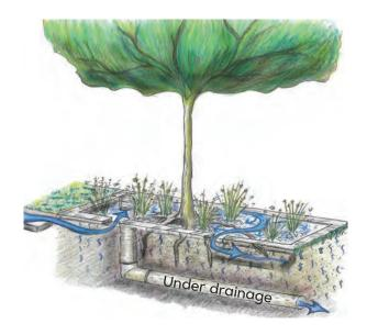
The above sketch illustrates a water smart street tree which utilises stormwater run-off from the road to irrigate the tree and ground cover planting.
